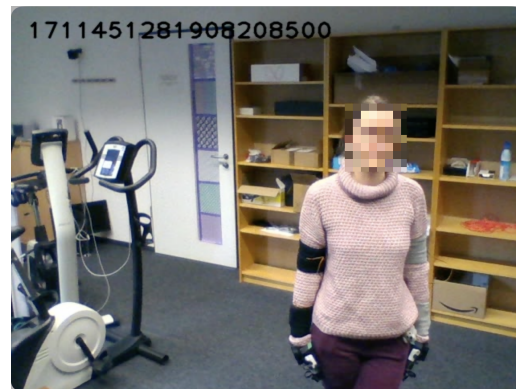
(b) Incorrect I-pose calibration with wrists rotated about the transverse axis (incorrect flexion/extension) and vertical axis (incorrect ulnar/radial abduction)
