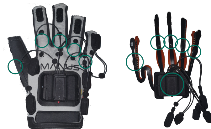
(a) Green circles indicate the IMUs (b) Brown stripes indicate the flex sensors
